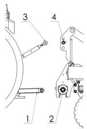
Figure 9. Connecting the unit to the tractor
