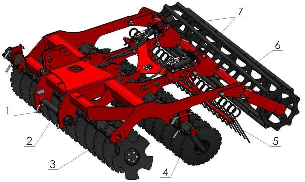
**Figure 5.** 1 – Lower link beam, 2 – Unit frame, 3 – Disc cutter, 4 – Outer disc support, 5 – Scraper beam, 6 – Shaft, 7 – Working depth adjustment.
