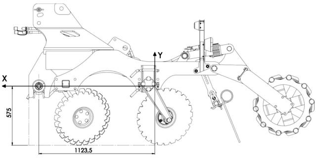
Figure 15. Position of the unit's centre of gravity - depending on the shaft used
