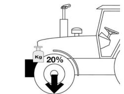
Figure 13. Minimum front axle load of the tractor
