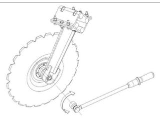
**Figure 11.** Tightening torque for the disc blade hub
