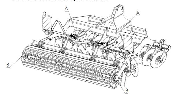
**Figure 12.** Lubrication of the unit: A - Shaft actuator, B - Shaft bearing assemblies.
