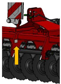
Figure 1. Location of the rating plate on the machine
