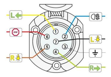
Figure 8. Diagram of the electrical plug connection
