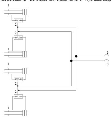
Figure 7. Hydraulic system diagram for U740/50: 1 - Shaft actuator, 2 - Controlled twin check valve, 3 - Hydraulic coupling.
