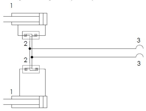
**Figure 6.** Hydraulic system diagram for U740/25, U740/30, U740/35, U740: 1 - Shaft actuator, 2 - Controlled twin check valve, 3 - Hydraulic coupling.
