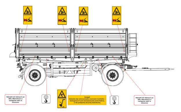
Fig. 8 The arrangement of the pictograms on the boards of the trailer – left side
