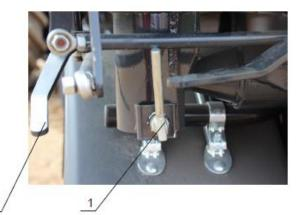
Fig. 17 The locks on the sideboards of the body.
