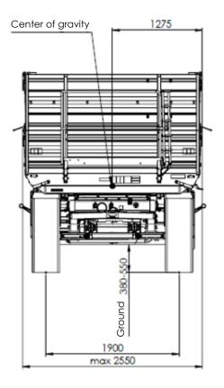
Fig. 9 Dimensions of the T739A trailer – front view
