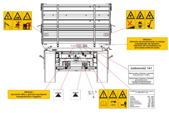
Fig. 5 The arrangement of the pictograms on the boards of the trailer - front
