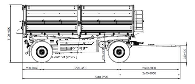
Fig. 10 Dimensions of the T739A trailer – side view
