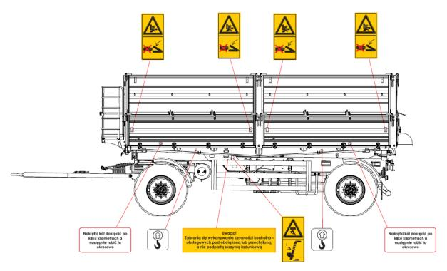
Fig. 7 The arrangement of the pictograms on the boards of the trailer – right side
