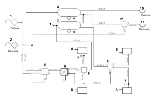
Fig. 16 Brake connection diagram – diaphragm actuators
