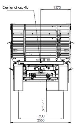
Fig. 11 Dimensions of the T958 trailer – front view
