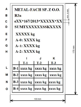
**Fig. 2** EU-approved trailer rating plate Key to the fields on the rating plate A – Manufacturer's name
