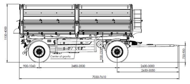
Fig. 12 Dimensions of the T958 trailer – side view
