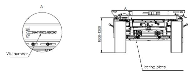
Fig. 1 Location of the rating plates and the VIN number on the machine
