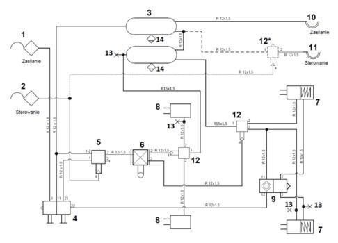
Fig. 15 Brake connection diagram – diaphragm spring actuators
