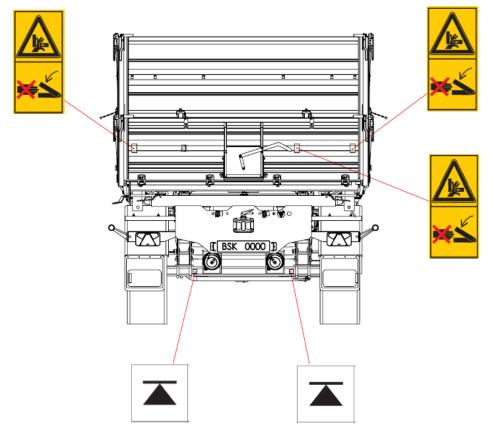
Fig. 6 The arrangement of the pictograms on the boards of the Trailer - rear
