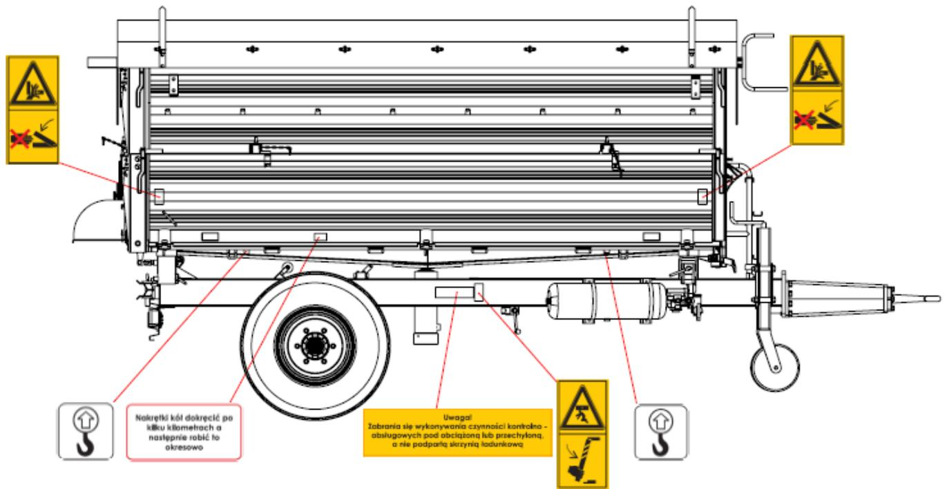
**Figure 6.** The arrangement of the pictograms on the boards of the Trailer – right side
