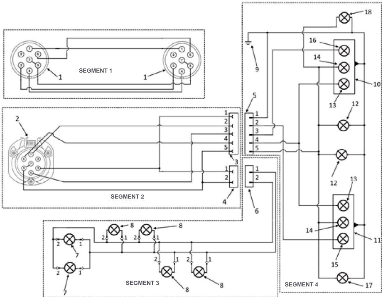
**Figure 12.** A diagram of the Trailer's electric system (version with side position lamps):
