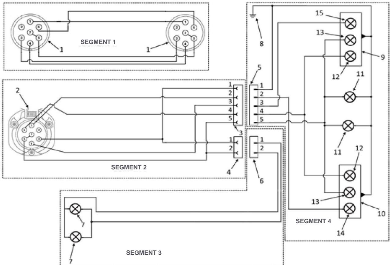
**Figure 11.** A diagram of the Trailer's electric system (basic version):
