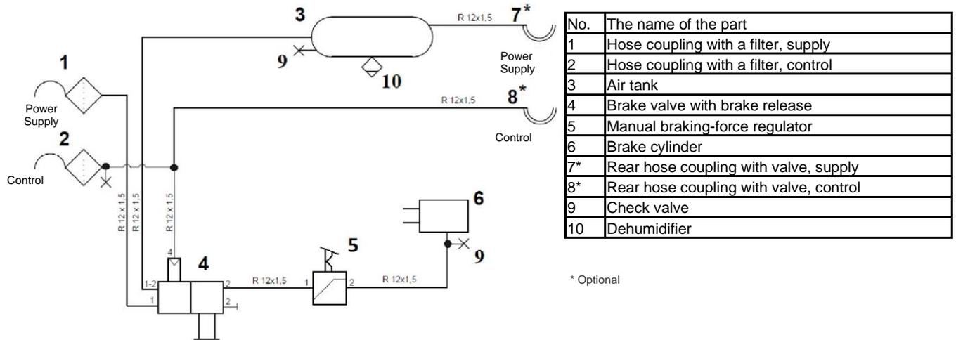
**Figure 14.** A diagram of a dual-line pneumatic braking system
