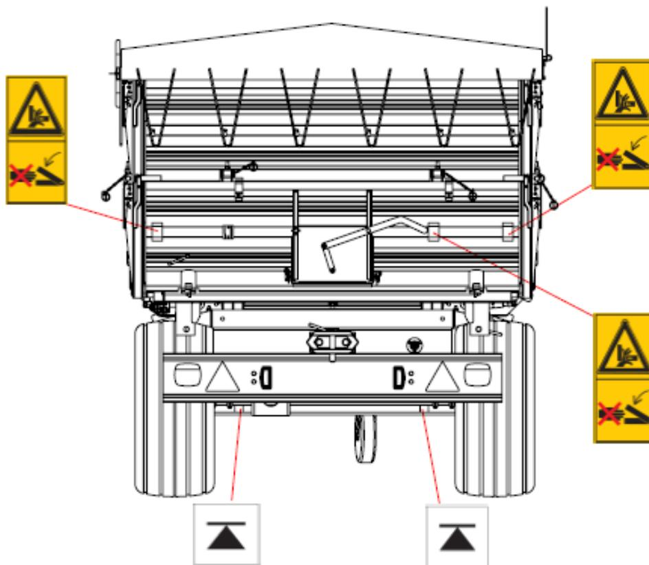
Figure 5. The arrangement of the pictograms on the boards of the Trailer - rear
