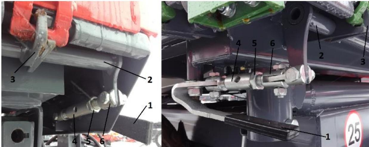
**Figure 18.** The locks on the sideboards of the load-carrying body:
