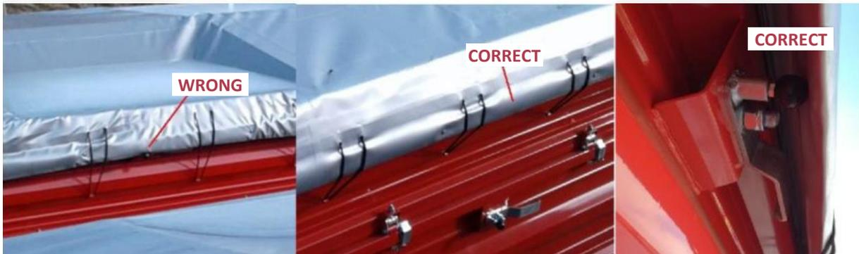
**Figure 3.** Correct tensioning of the tarpaulin cover
