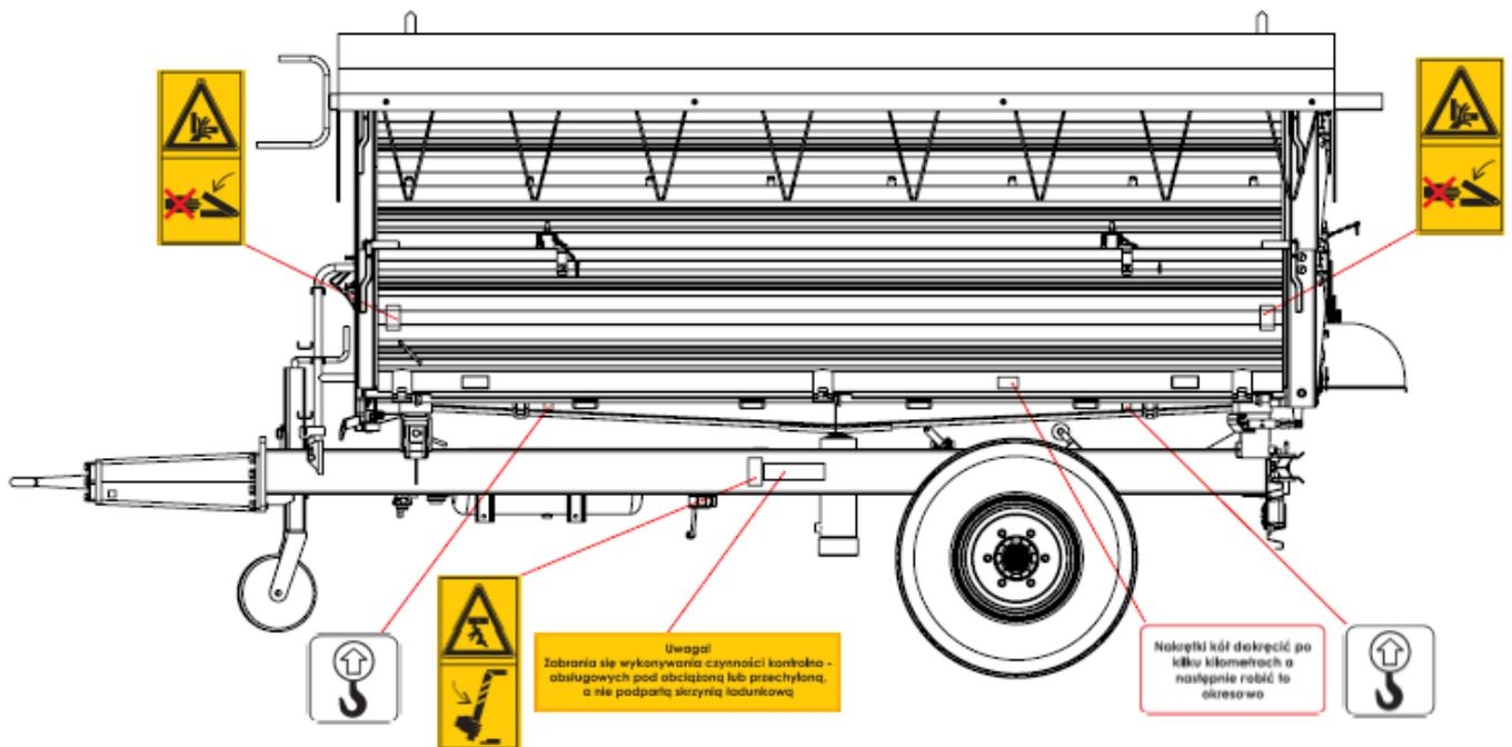
**Figure 7.** The arrangement of the pictograms on the boards of the Trailer – left side
