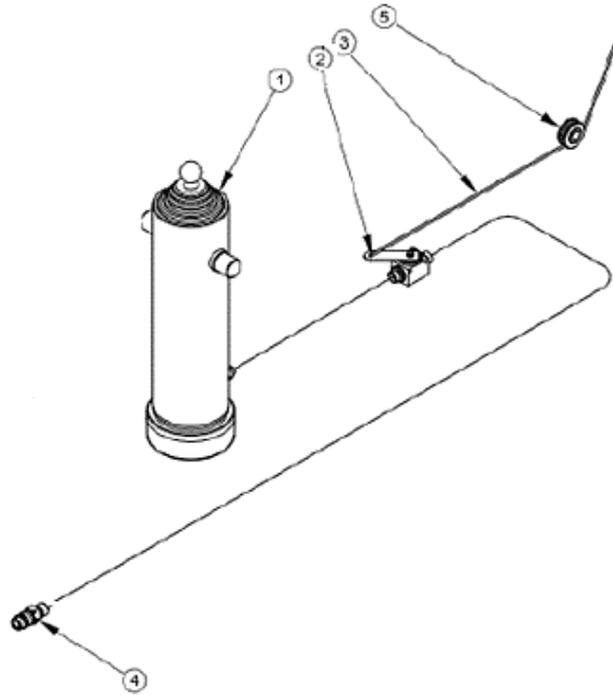
**Figure 10.** The diagram of the hydraulic system in the tilting mechanism of the Trailer's body:
