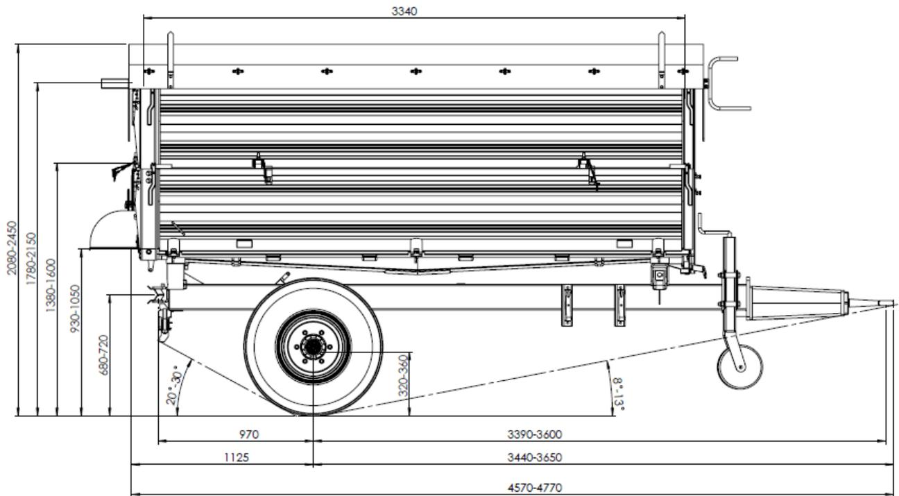
**Figure 9.** Dimensions of the Trailer – side view
