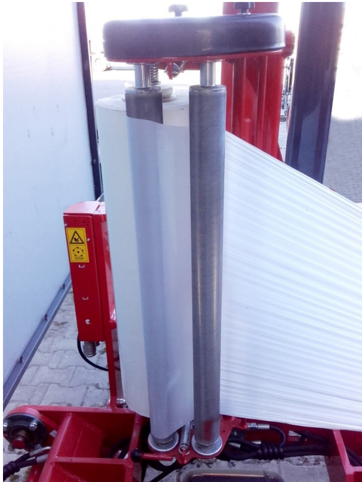
Figure 33. Correct installation of the foil in the feeder
