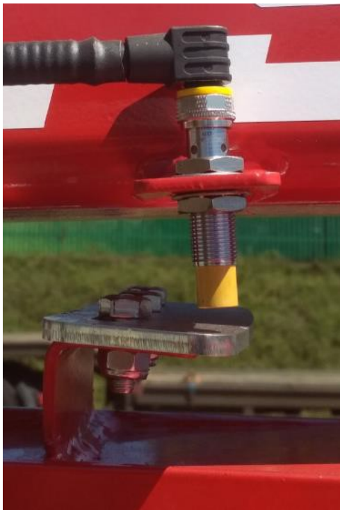
Figure 22. Inductive revolution sensor setting
