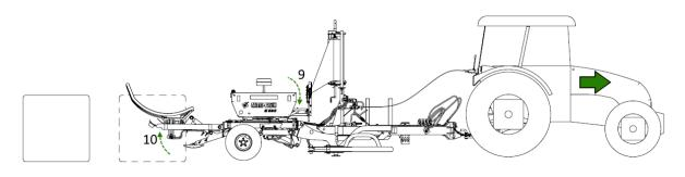
Figure 49. The service table and bale tipper being set to the servicing position
