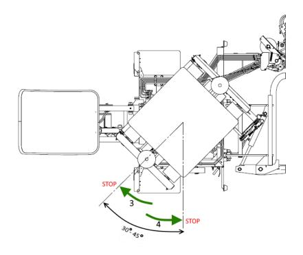
Figure 44. Stopping and locking the service table
