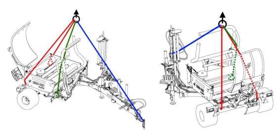
Figure 58. The suspension-sling attachment points on the Bale Wrapper
