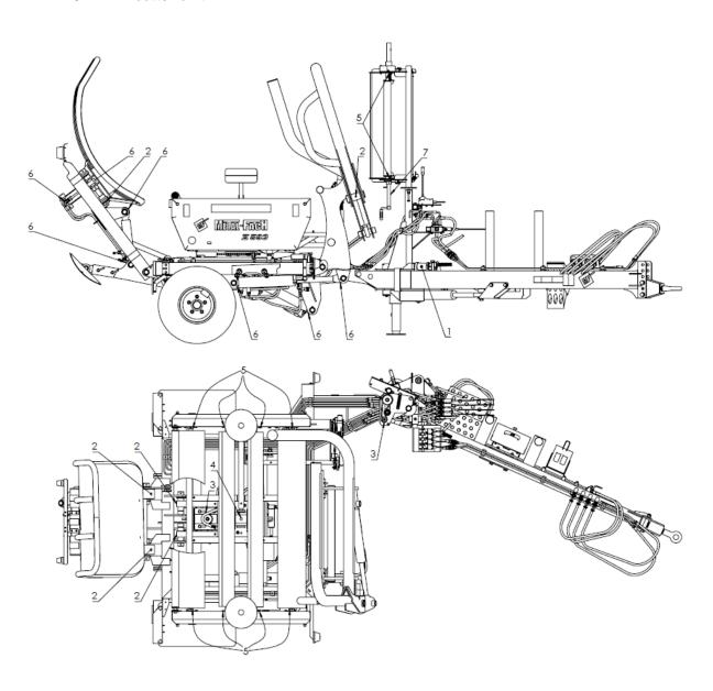
Figure 51. Lubrication points – top right-hand side view
