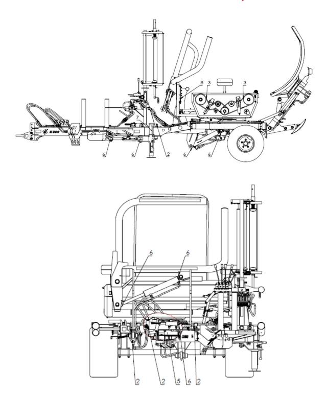
Figure 52. Lubrication points – front left-hand side view
