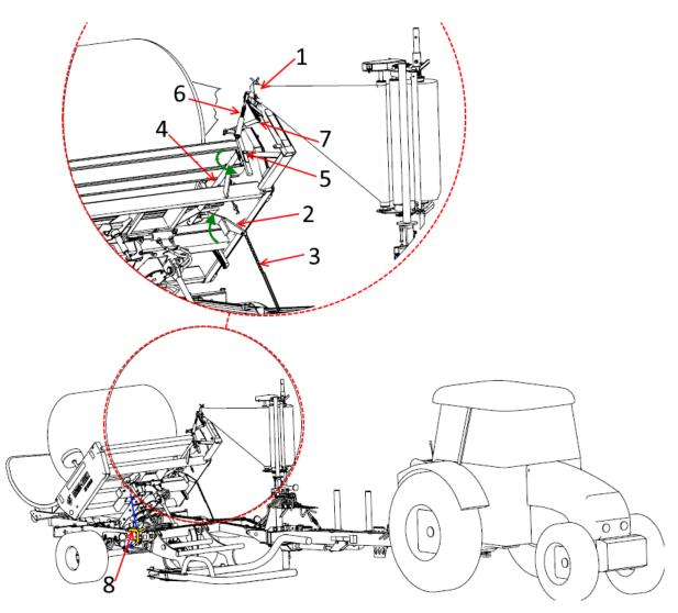
Figure 50. Grabbing and cutting the film
