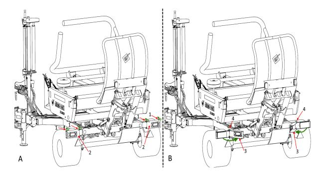
**Figure 56.** Lighting housings, A – service position, B – the transporting position
