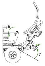
**Figure 54.** Setting the transporting position of the bale tipper's support foot
