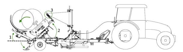
Figure 46. Raising the service table and the bale-tipper unit
