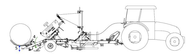
Figure 47. Lowering the tipper unit with a bale in the grab
