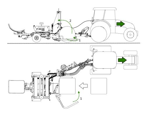
Figure 41. Bale-Wrapper position for bale loading
