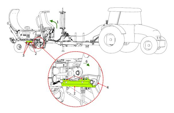
**Figure 55.** The loading arm's transporting lock
