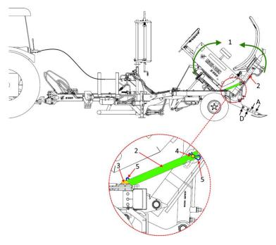
**Figure 53.** Locking the bale tipper in the transporting position
