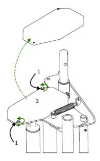
Figure 32. Dismount the guard of the feeder-chain drive
