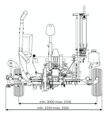
Figure 5. Wrapper dimensions – front
