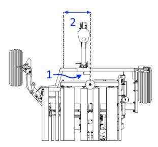
Figure 26. Adjusting the bale tipper
