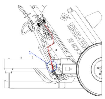
Figure 41. The location of the wire-length adjustment
