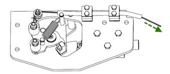
Film-cutter activation module – the closed-cutter position Figure 40.
