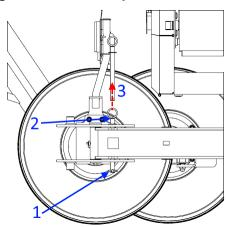
Figure 21. Unlocking the axle shaft's position
