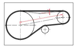
Figure 28. Chain-tension adjustment – determining a chain bend: f – chain-bend value, L – distance between the sprocket-centre lines  $f = 0.1 \times L$
