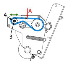
Figure 33. Adjust the tension of the feeder-drive chain
