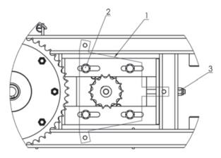
Figure 29. Drive-chain adjustment 1 – Chain guard, 2 – M12 nuts, 3 – Chain-tensioner bolt
