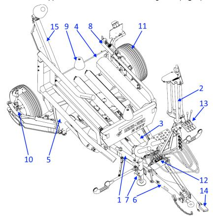
Wrapper design 1 – Main frame, 2 – Film feeder, 3 – Moving frame, 4 – Rotary frame, 5 Figure 4. - Loading arm, 6 - Drawbar, 7 - Support foot, 8 - Cutting unit, 9 - Side cone, 10 - Rotating axle shaft, 11 - Fixed-axle shaft, 12 - Hydraulic manifold, 13 - Control levers 14 - L-02 Counter, 15 - Bale tipper
