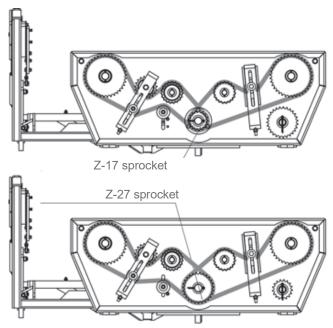
Figure 34. The sprockets of the roller-drive chains
