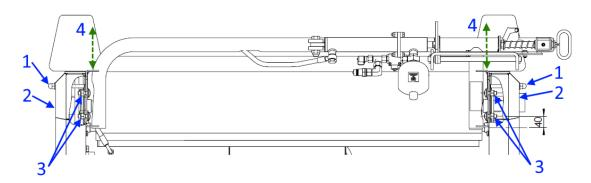
Figure 39. Adjusting the cutter height
