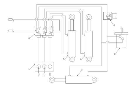
Figure 14. The hydraulic system of the Z577 Bale Wrapper with mechanical film cutter
