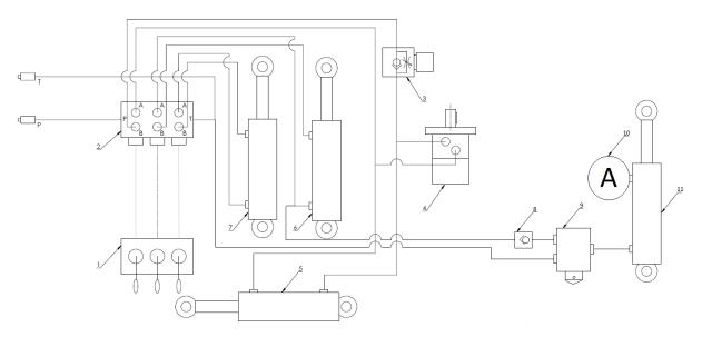
Figure 13. The hydraulic system of the Z577 Bale Wrapper with hydraulic film cutter
