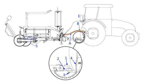
Figure 9. Connecting the hitch and drive of the Bale Wrapper
