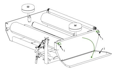
Figure 30. Dismount the guard of the roller-drive chain
