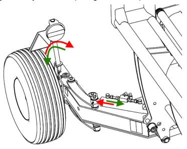
Figure 25. The hydraulic shifting of the ground wheel
