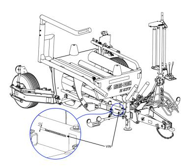
Figure 3. Location of the VIN on the machine
