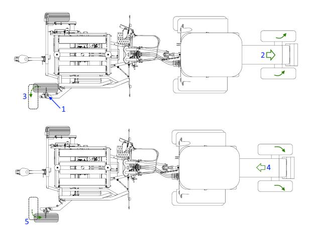
Figure 23. Shifting the drawbar from the transporting to working position
