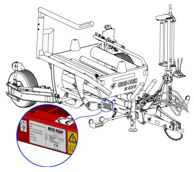
Figure 2. Location of the rating plate on the machine
