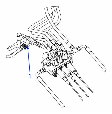
Figure 36. The location of the adjustment valve for the service-table lock
