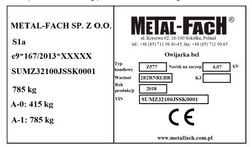
Figure 1. Example of a rating plate
