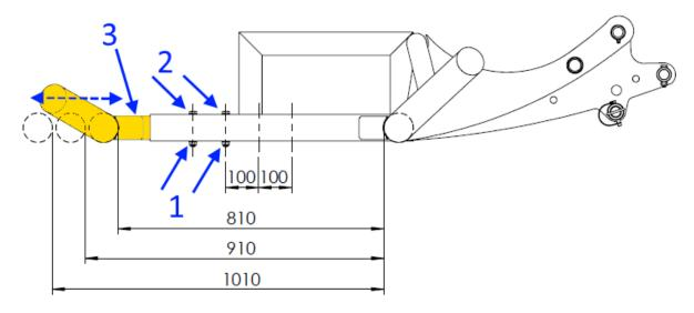
Figure 27. Changing the loading arm's width
