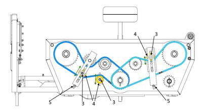
Figure 31. Adjust the tension of the roller-drive chains
