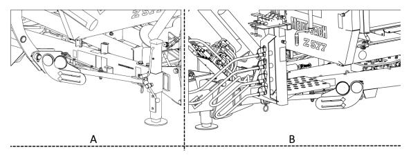
Figure 44. The front-lighting-service position A – right side, B – left side
