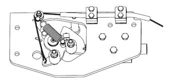
Figure 42. The film-cutter activation module – the open-cutter position
