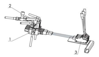
Figure 15. The hydraulic system 1 – 3-section manifold, 2 – Valve, 3 – Control levers
