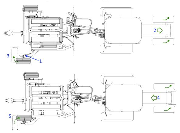
Figure 24. Shifting the drawbar from the working to transporting position
