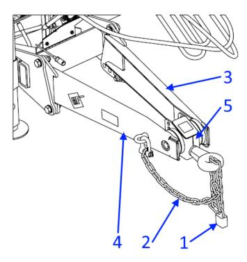
Figure 10. Drawbar components
