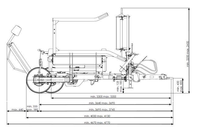
Figure 6. Wrapper dimensions - side
