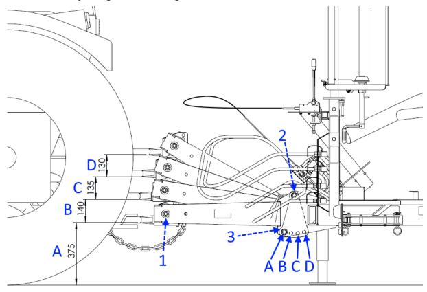
Figure 20. Adjusting the hitch height
