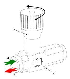
Figure 35. Throttle/non-return valve, 1 – Valve handwheel, 2 – Valve shell marked for the throttling direction, 3 – Throttled-flow direction, 4 – Free-flow direction
