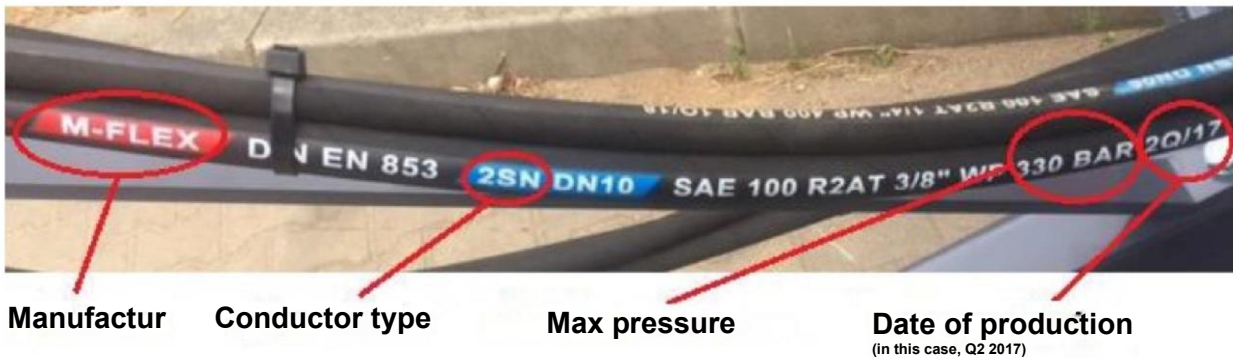
Figure 38. Marking of the hydraulic lines
