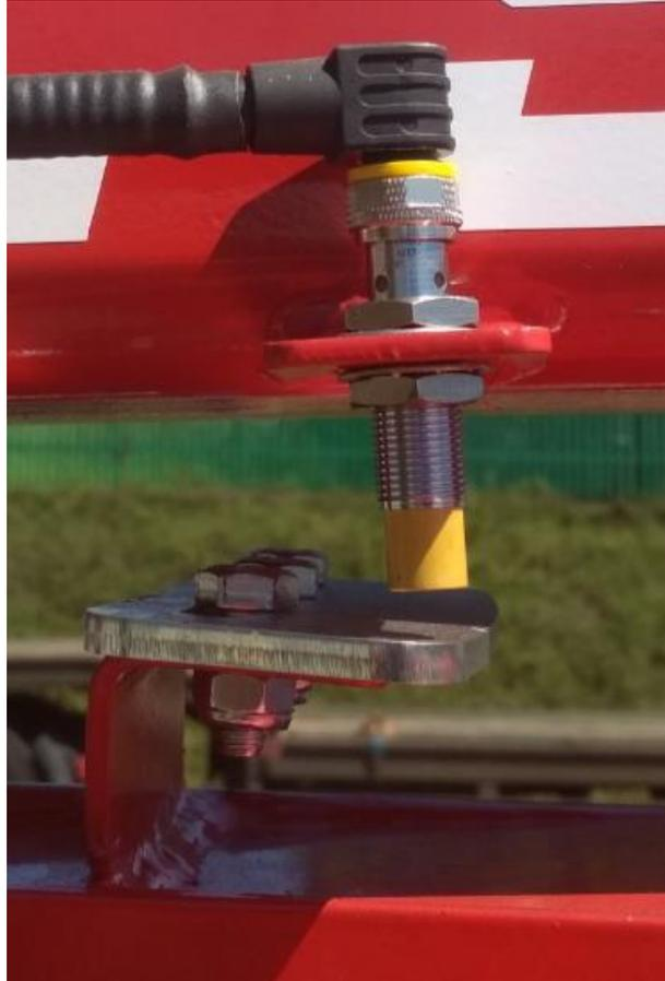
**Figure 22.** Inductive revolution sensor setting
