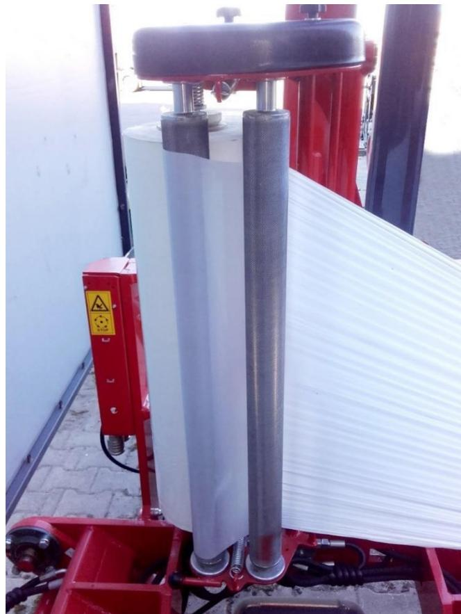
**Figure 33.** Correct installation of the film in the feeder
