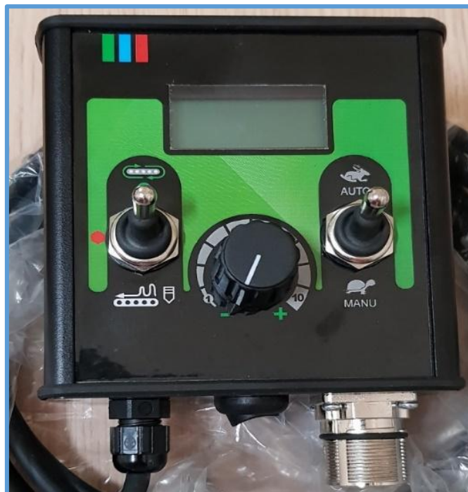
Figure 29. Control panel for adjusting the speed of the floor conveyor by means of a potentiometer – control knob (optional accessory).
