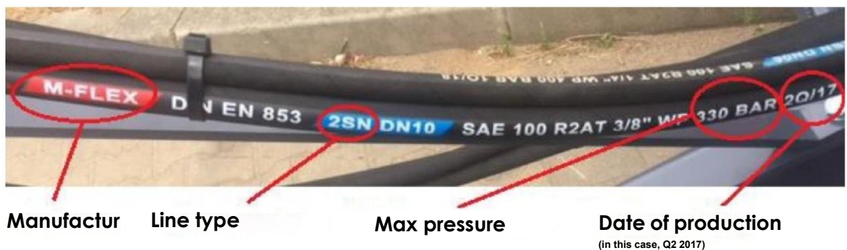
Figure 23. Marking on hydraulic lines
