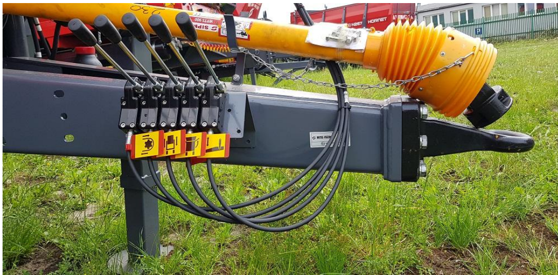
Figure 25. Pictograms for the control levers of the distributor (distributor control is optional)
