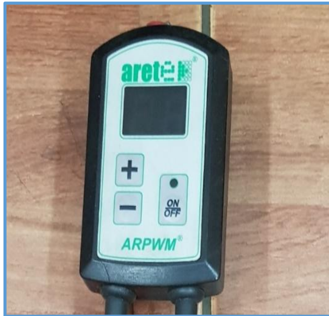
Figure 28. Control panel for adjusting the speed of the floor conveyor with "+/-" buttons (optional equipment).
