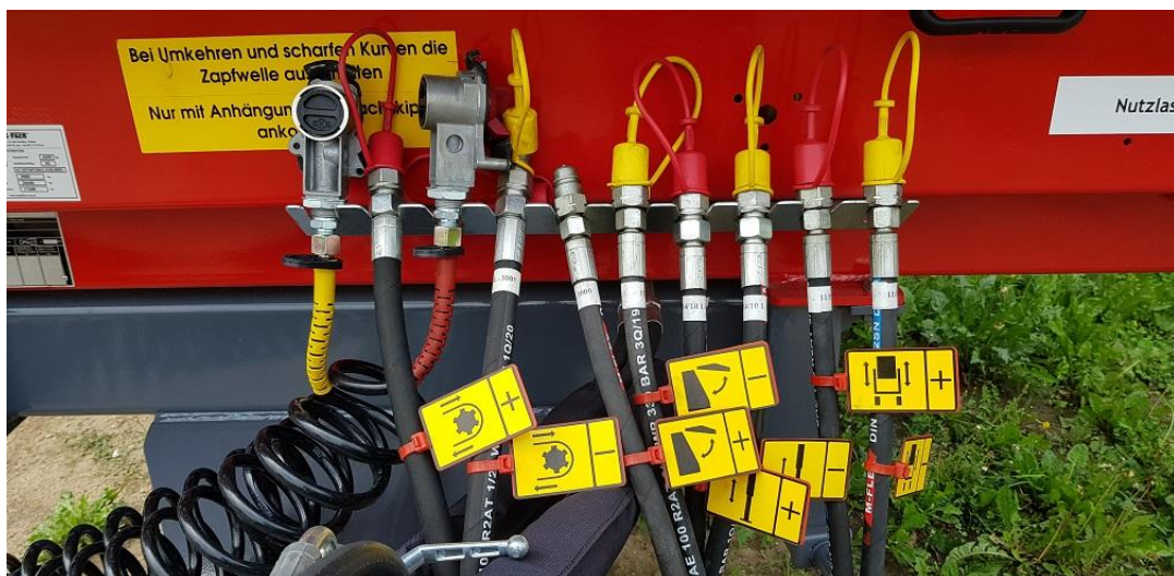
Figure 24. Pictograms on the hydraulic connectors for easier connection to the tractor
