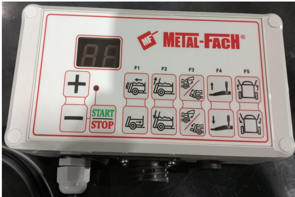
Figure 30. Hydraulic control panel,
