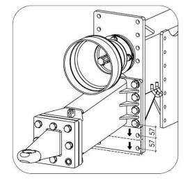
Figure 19. Adjusting the hitch height
