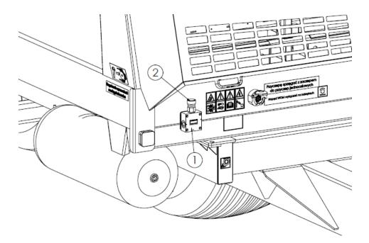
**Figure 24.** Adjusting the travel speed of the floor conveyor: 1 - oil flow regulator, 2 - regulator knob
