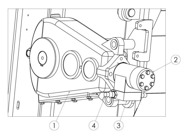
**Figure 26.** The drive of the floor conveyor 1 – gearbox, 2 – hydraulic motor, 3 – overload valve, 4 – valve seal
