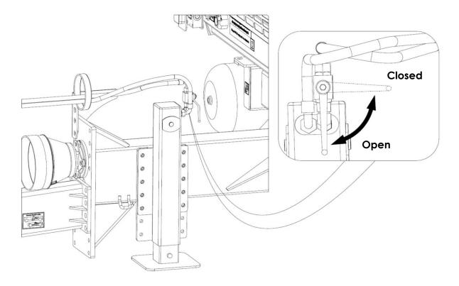
Figure 20. Hydraulic valve to control (shut off) the hydraulic parking jack
