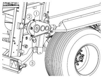
**Figure 30.** Oil level control points in the floor conveyor's transmission: 1 – oil filler (vent), 2 – oil-level sight glass, 3 – drain plug
