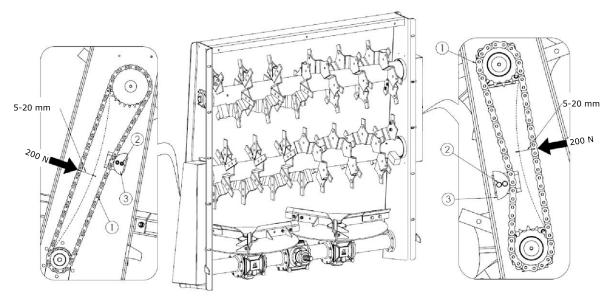
Figure 29. Tensioning the beater unit chains
