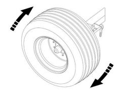
Figure 41. Checking wheel bearing play
