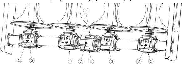
Figure 32. Oil level control points in the 4-auger adapter gearbox 1 - oil filler (vent), 2 - oil-level sight glass, 3 - drain plugs
