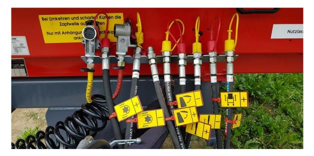
Figure 22. Pictograms on the hydraulic connectors for easier connection to the tractor (standard)
