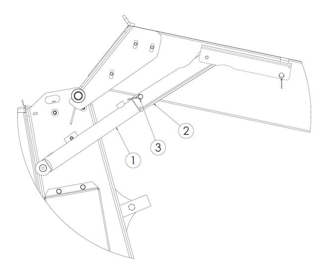
Figure 45. Locks for securing the cylinders
