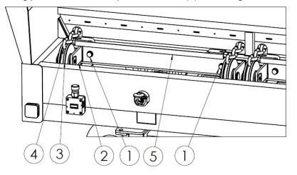
**Figure 27.** Tensioning the chains of the floor conveyor: 1 – adjusting screw, 2 – tensioner slide, 3 – tensioner pulley, 4 – conveyor chain, 5 – conveyor bar
