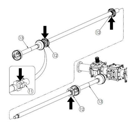
Figure 34. Spreader lubrication points
