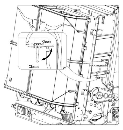
Figure 25. Hydraulic valve for locking the beater unit shield
