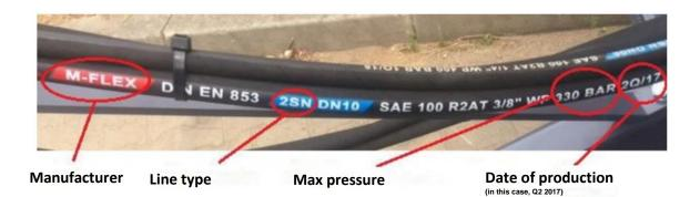
Figure 21. Marking of the hydraulic lines
