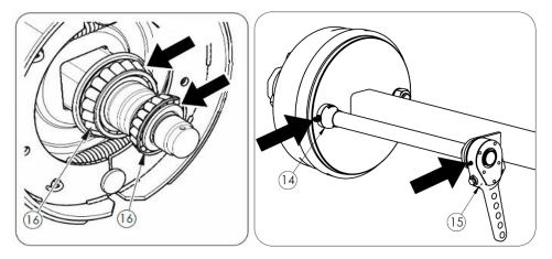
Figure 35. Spreader lubrication points
