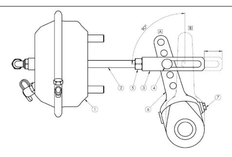
Figure 43. Adjustment of the parking brake
