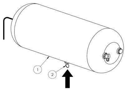
Figure 40. Draining the air tank: 1 - air tank, 2 - drain valve
