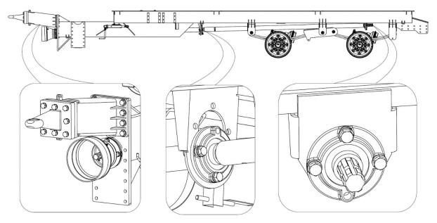
Figure 17. Position suitable for connection to the tractor's lower hitch
