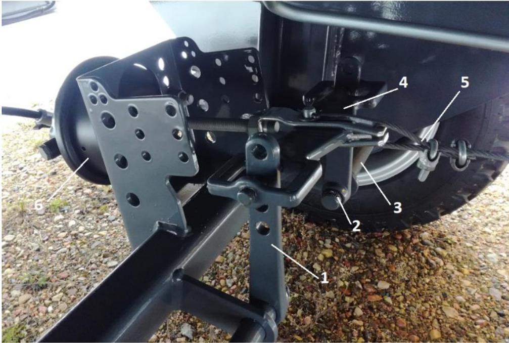
**Figure 17.** The components of the brake system:
