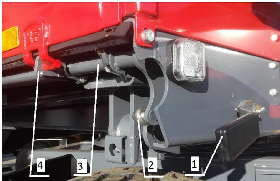
**Fig. 19.** The locks on the sideboards of the load-carrying body: 1 – central lever of the bottom locks, 2 – lock adjustment mechanism, 3 – central lock shaft, 4 – lock
