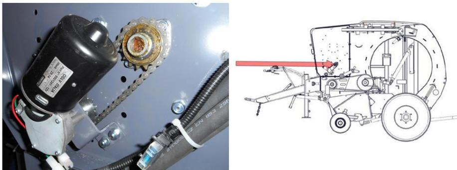
**Figure 32.** Lubricating the net chain
