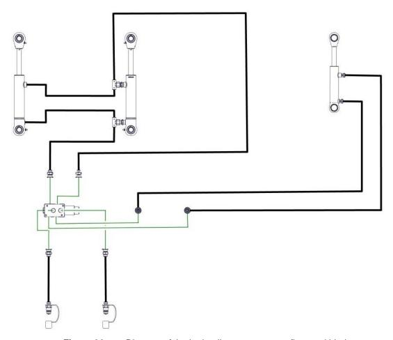
**Figure 36.** Diagram of the hydraulic system – rotor floor and blades
