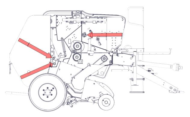
Figure 30. Lubrication points (right side)
