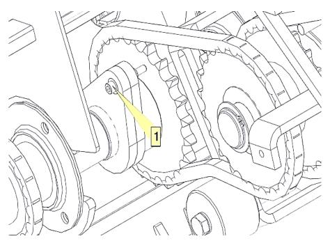
Figure 22. Replacing the locking bolt
