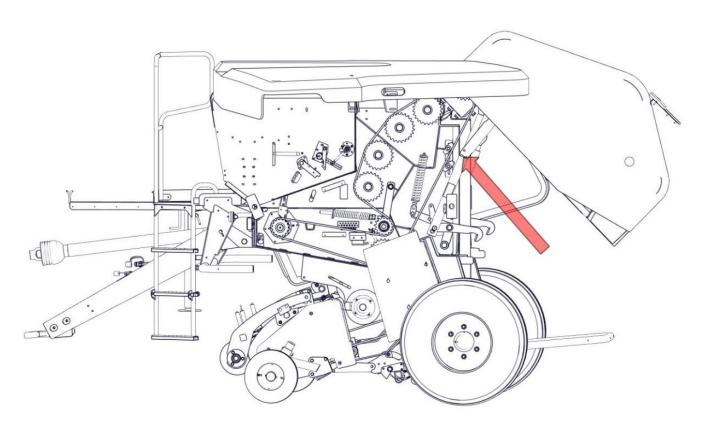
Figure 9. Locks for securing the cylinders
