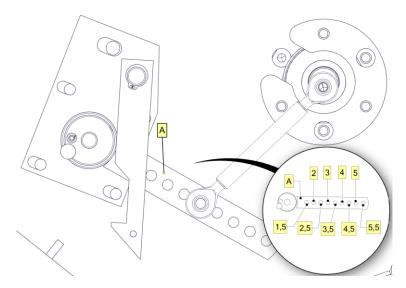
Figure 24. Net binding device adjustment
