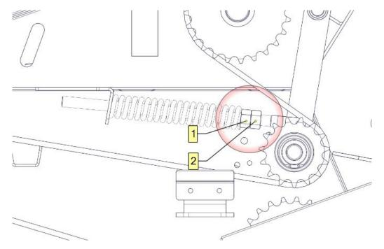
**Figure 13.** Adjusting the automatic chain tensioners
