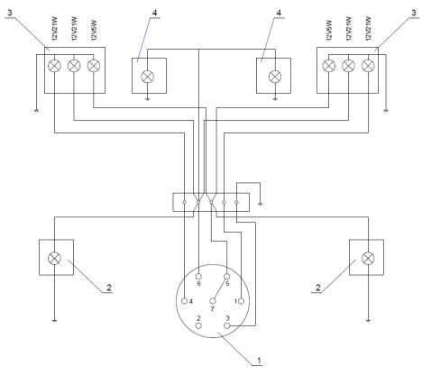
Figure 37. Wiring Diagram (1 - connection plug, 2 - head light, 3 - tail light, 4 - licence plate light)
