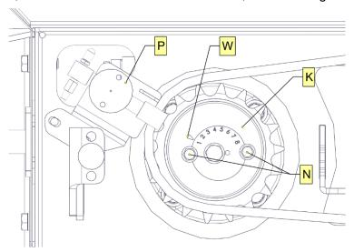
Figure 31. Adjusting the oil amount in the automatic lubrication system
