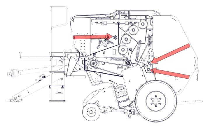
Figure 29. Lubrication points (left side)
