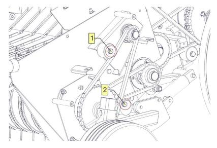
Figure 14. Adjusting the tension of the pick-up chains
