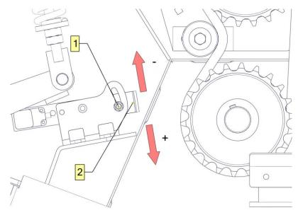
Figure 25. Adjusting the degree of compaction
