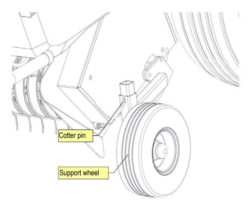
Figure 10. Adjusting working height of the pick-up
