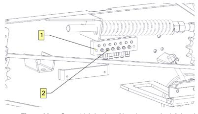
Figure 33. Central lubrication of bearings on the left-hand side of the baler
