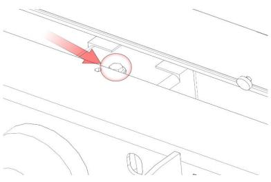
Figure 27. Oil level in the gearbox
