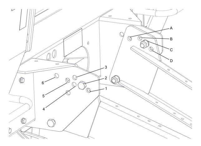
Figure 3. Setting the drawbar height
