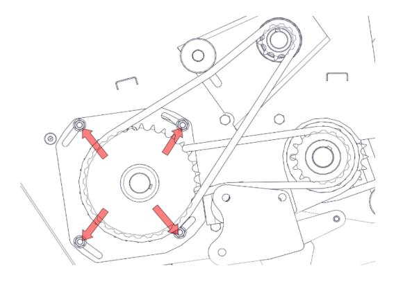
Figure 20. Pick-up cam adjustment
