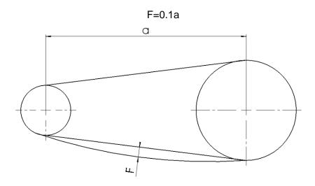
Figure 12. Chain tension
