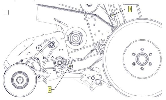
Figure 15. Adjusting the chain tension on the left-hand side of the baler
