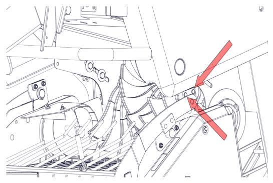
Figure 8. Windrow clamp dismantling
