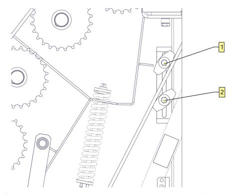
Figure 16. Adjusting the chain guiding performance on the left-hand side of the baler
