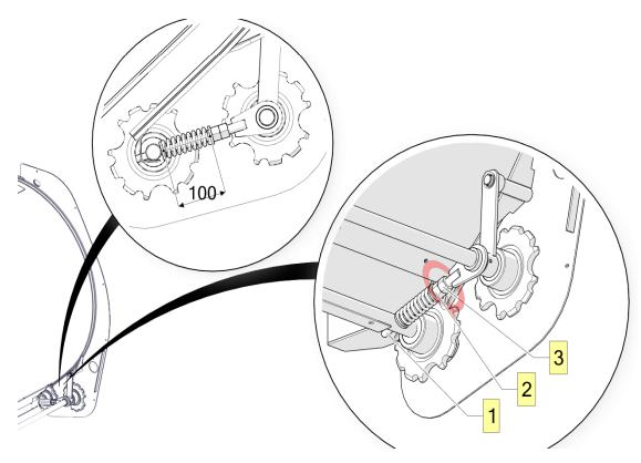
Figure 19. Adjusting the tension of the chain and rod conveyor set
