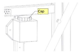
Figure 32. Oil tank of the automatic chain lubrication system
