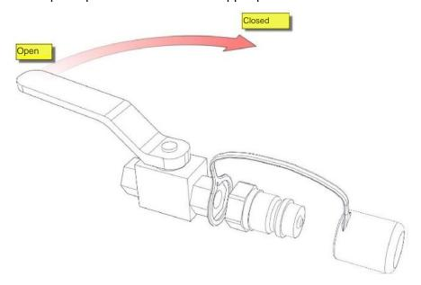
Figure 6. Cut-off valve
