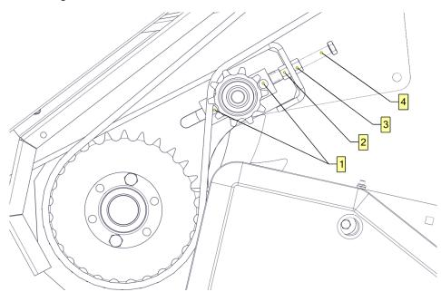
Figure 18. Adjusting the tension of the rotor chain
