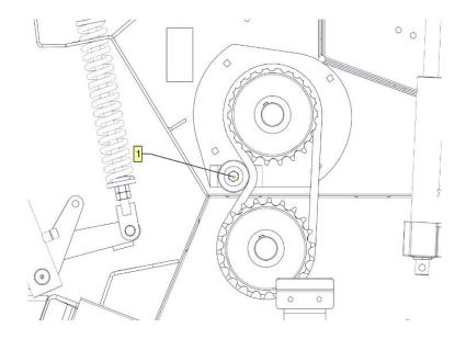
Figure 17. Adjusting the chain tension on the right-hand side of the baler
