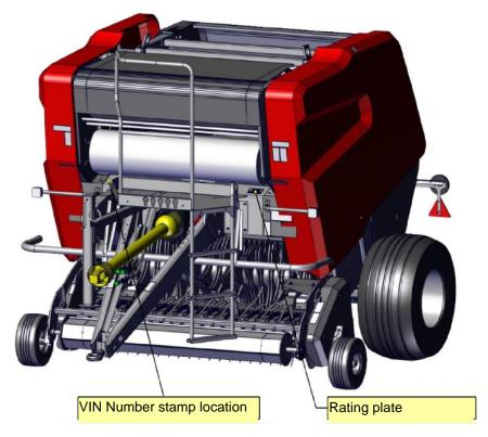
The location of the nameplate and the VIN on the machine Figure 2.
